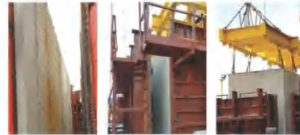
Demoulding and hoist up of the modules
